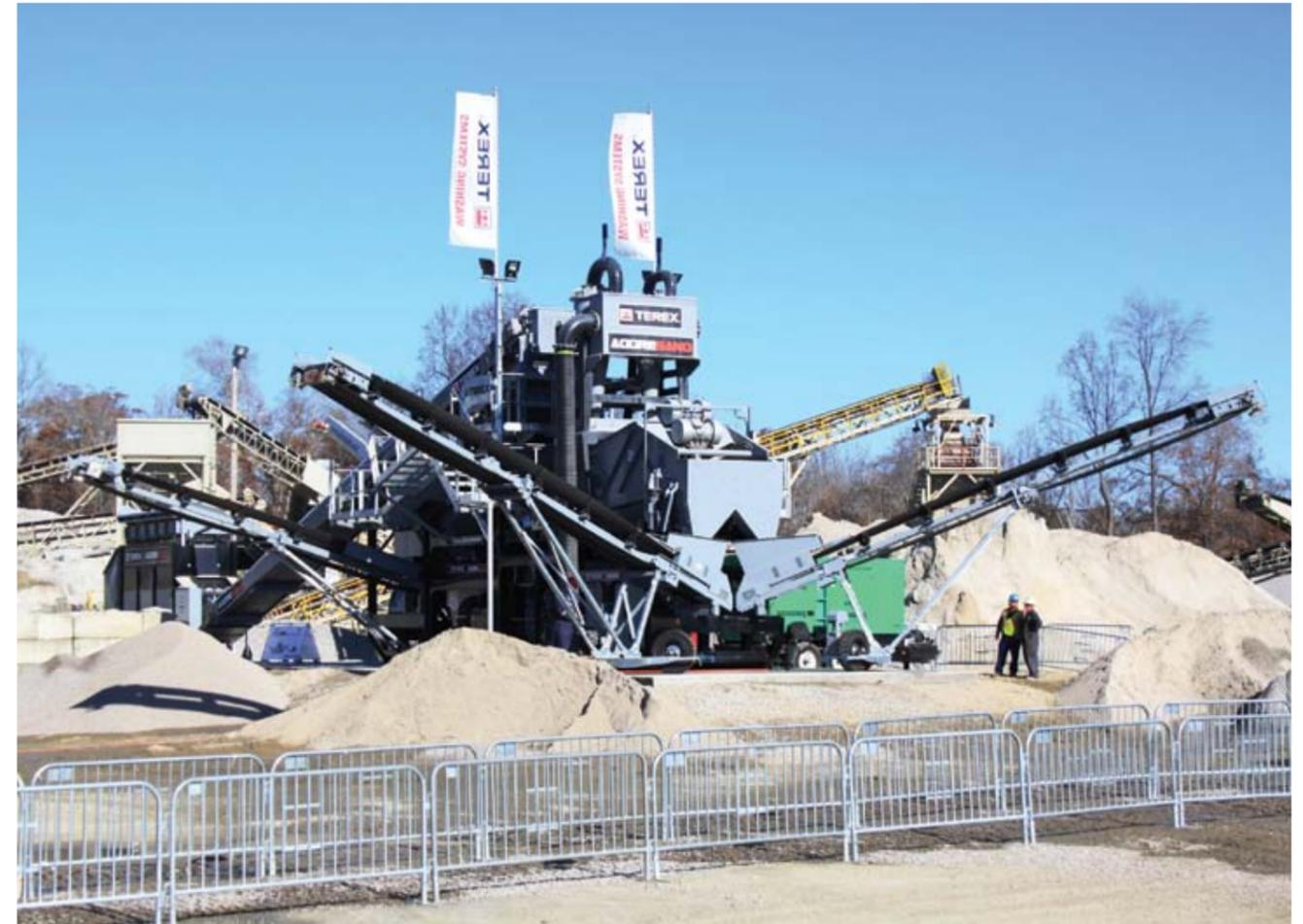
Aggresand 165, High Capacity Sand Plant, USA
