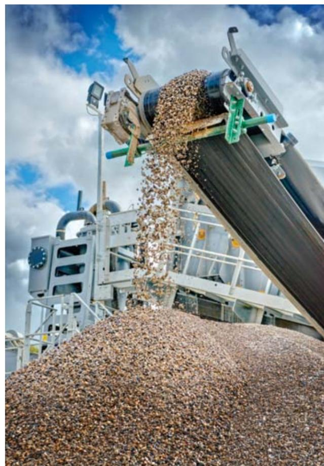
Integral Aggregate Stockpiling Conveyors
