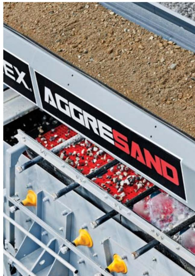
Aggregate Screen Fitted with Isolated Spraybars
