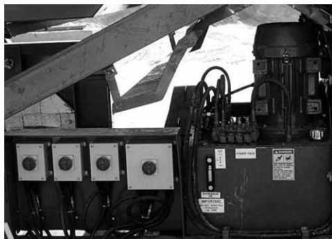
Integrated electric powerpack for bucket wheel speed adjustment
