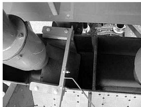
Movable chute to allocate fine material to the coarse product
