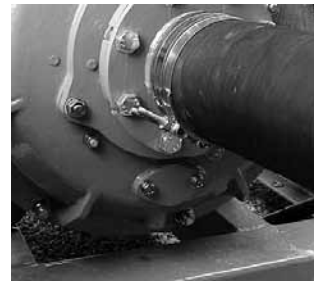
Pump drain for cold climate applications
