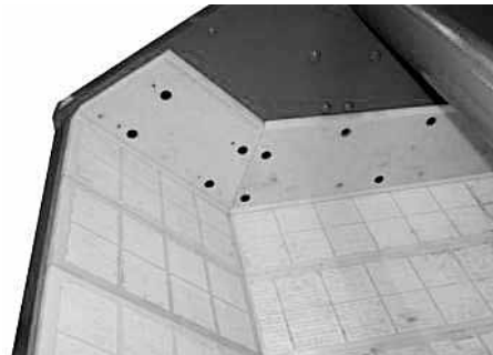
Sloped back panel for maximum water removal
