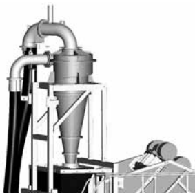
Rubber lined sealed slurry transfer pipe complete with heavy duty clamps
