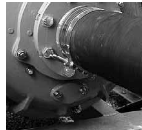
Pump drain for cold climate applications
