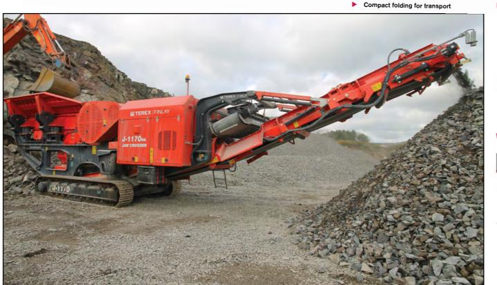
Machine weight: 48,900kg (107,806lbs) (with HA chamber, standard VGF, standard main conveyor, magnet and by-pass conveyor)
