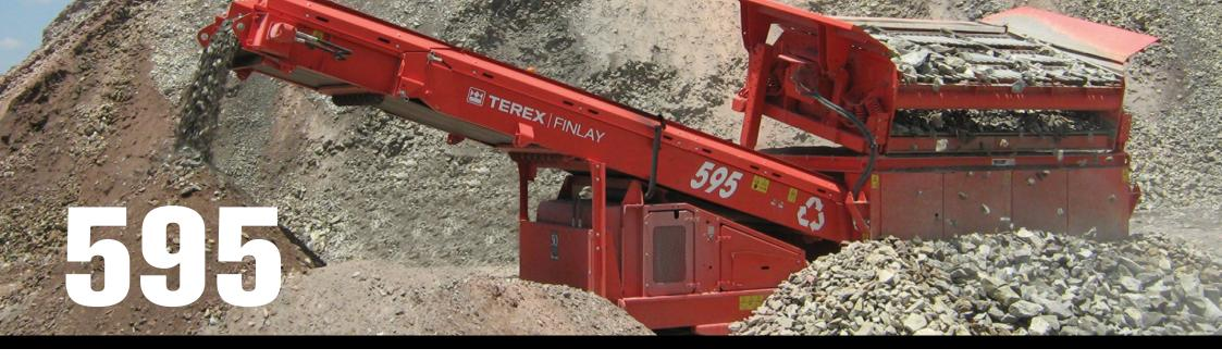
The Terex Finlay 595 Hydratrak is a self contained high capacity mobile scalping unit. Designed and constructed to the highest specification, the 595 can withstand the toughest of applications from waste reclamation projects to quarry face and demolition environments, special features include a heavy duty twin deck vibrating grid, remote control movement and a tracked undercarriage.
