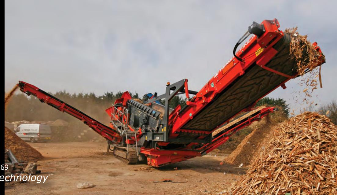
The new Terex Finlay 883+ Spaleck is the ultimate in mobile screening and separation technology. At the heart of the machine is the 2 deck German designed and constructed high performance screenbox.
