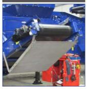
Magnetic Head Drum provides additional revenue by extracting ferrous metal from the waste stream
