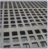
Provides additional throw & reduces the chance of plugging. Suitable for sticky and wet materials
