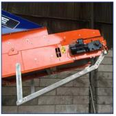
Magnetic Head Drum provides additional revenue by extracting ferrous metal from the lights material
