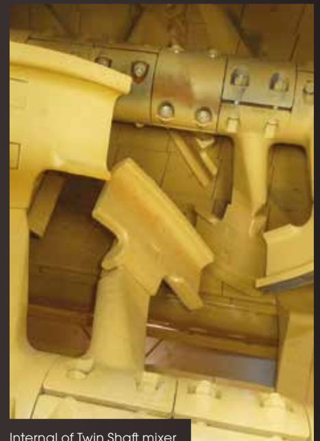
Internal of Twin Shaft mixer
