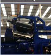
Overband magnet fitted to collection conveyor to extract ferrous metal
