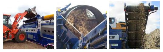
The TR622 Trommel combines high production rates with ease of use in a robust, portable and versatile screening plant that is ideal for applications such as top soil, recycling, composting and is proven in construction and demolition waste.
