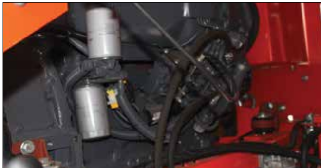
Engine: Tier 4i/ Stage 3B Deutz D914 L04i
