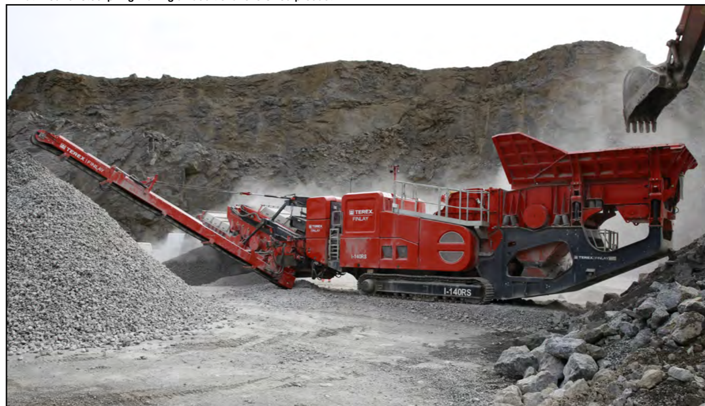
Machine weight: 71,200Kg (156,969lbs) *est (with Prescreen, by-pass conveyor, underpan & magnet options)
