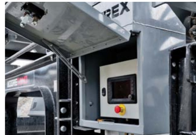
Cutting Edge Control Panel
