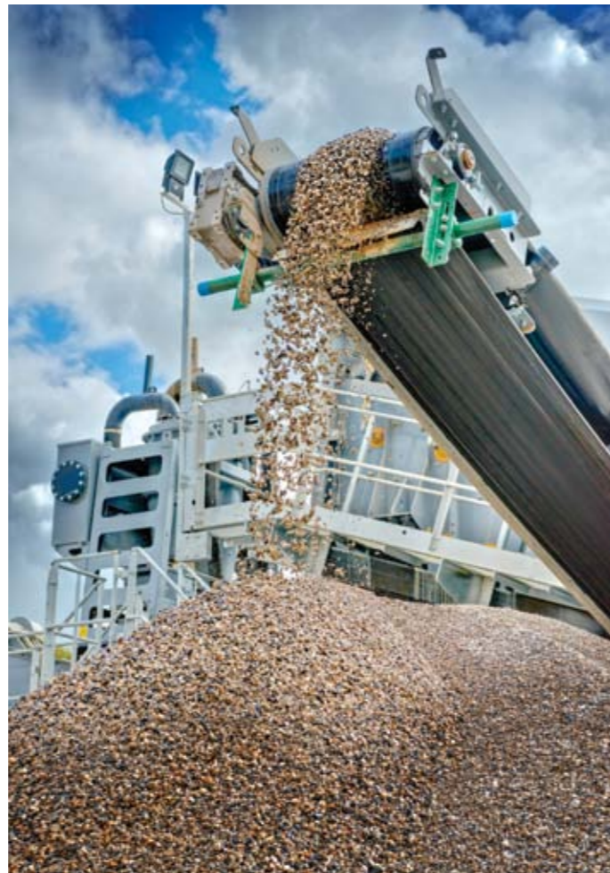
Integral Aggregate Stockpiling Conveyors
